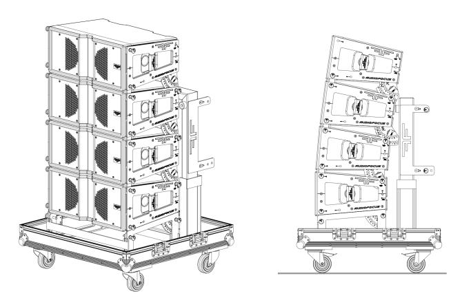
One of the benefits on an AUDIOFOCUS supplied ARES8 flight case is the ability to pre configure your cabinets angle before leaving the warehouse, further minimising on-site rigging time.
