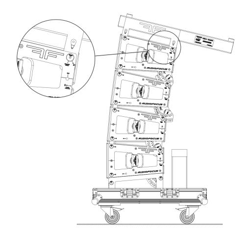
Bottom ARES8 pin has to be remove with a minimal hoist tension.
