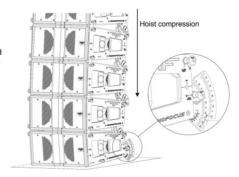
Last step is to lift the ARES8 line source to the proper height as calculated by Easefocus. The preset and level can be adjust easily while the cabinets are at human height. Each cabinet sound and connection can also be check at this time.
