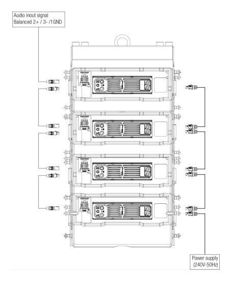
Passive version only have the speakon connector on the back. As it is a two voice speaker, a 4P speakon connector is needed (1+/1- low; 2+/2-high). Powersoft Armonia hold all ARES8 presets as in Powersoft X series or Canalli amplifier. One output can drive up to heigh Serial version of ARES8p and two Parallels version of ARES8p. Use 2.5mm<sup>2</sup> speaker cable.
