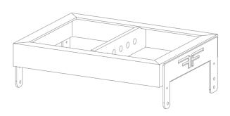
The over-hat is suitable for a limit of 6 Ares8 on top of MTsub218mkII, depending on tilt angle
