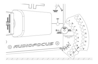
Also, easiest way to trigger the angle is compression method by using bottom ARES8 in floor position.
